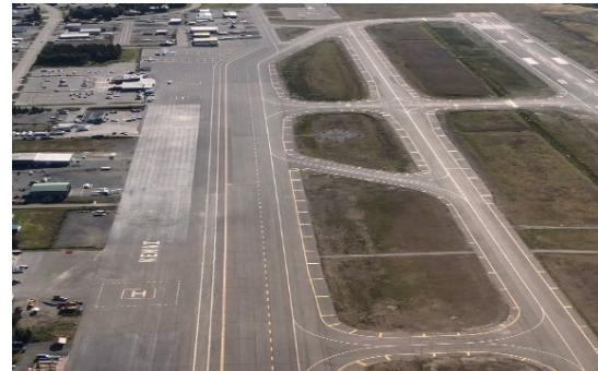
Details: This project will rehabilitate runway taxiways A, B, C, D, E, K, L, and M to current standards. The work will involve milling the existing taxiways and placing new asphalt surfaces, markings, and lighting. Design funds of \$650,000 were forward funded already for this project. This appropriation would be remaining match needed for construction.
