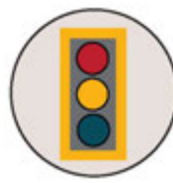
BACKPLATES WITH RETRO-REFLECTIVE BORDERS
