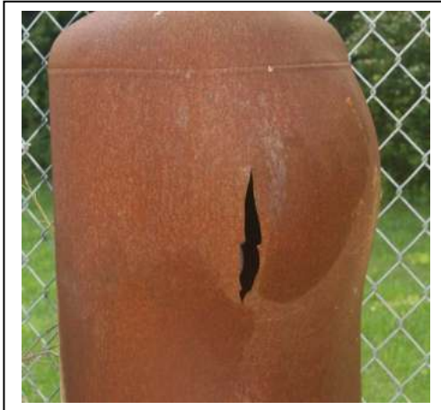
Fire Damaged, bulged Cylinder
