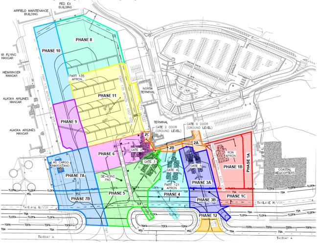
As of September 1, the passenger boarding bridges (PBB) at Gate 2, Gate 4 and Gate 5 are in use. The Gate 3 apron (Phase 5 work area) remains closed to all aircraft while Alaska Airlines / Roger Hickel continue to work on the installation of their new PBB. The new RON (gate 6) remains available and is being used on an as-needed basis.
