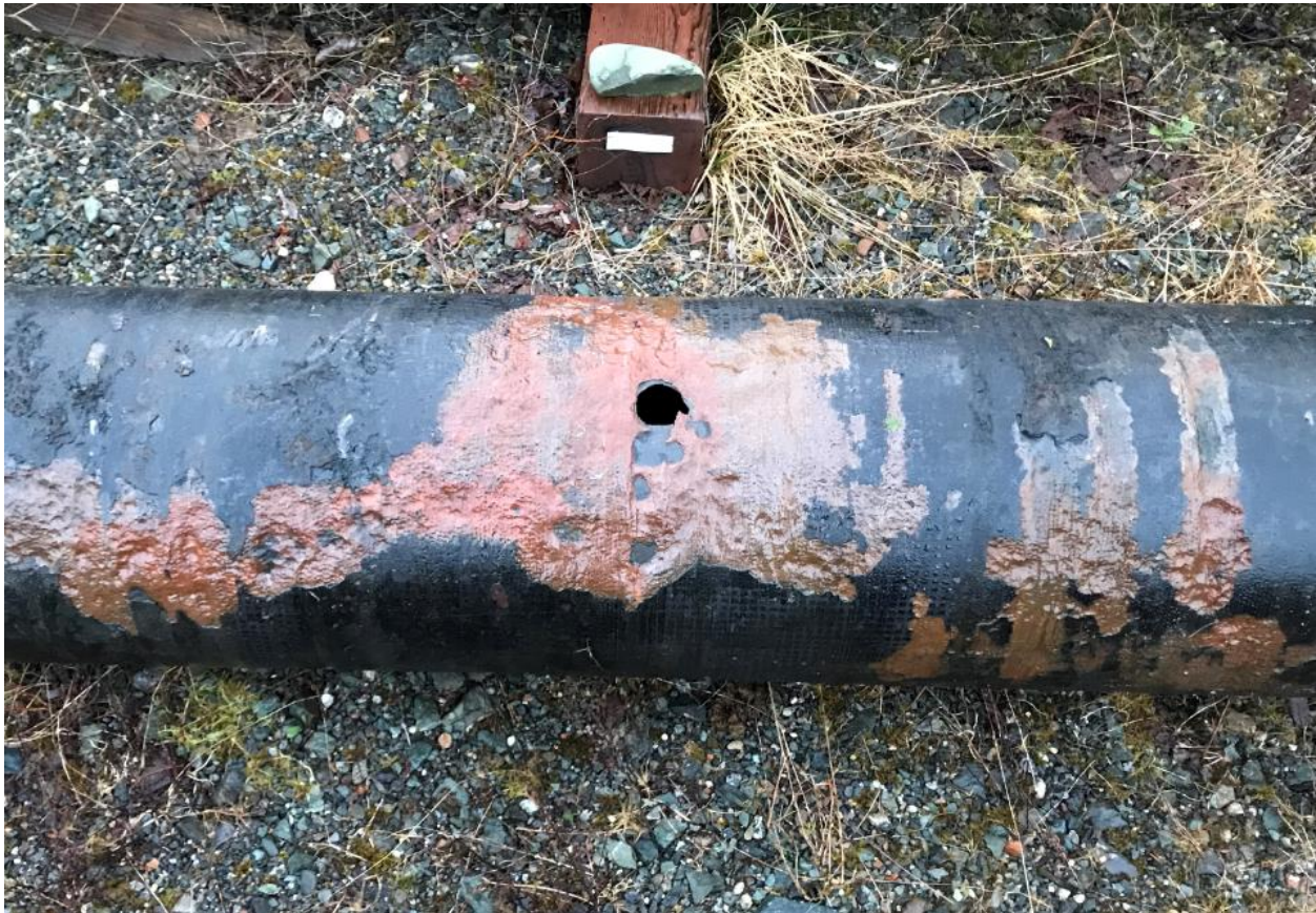
Failed water pipe from Lena Loop – CBJ Water Utility Staff photo
