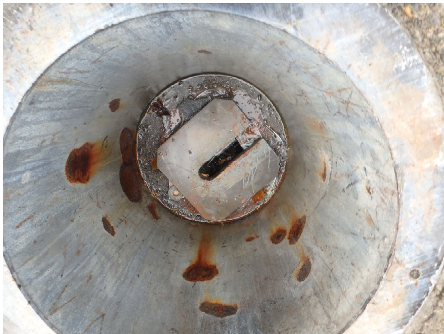
Photo 6. Inside of hawse pipe with chain keeper
