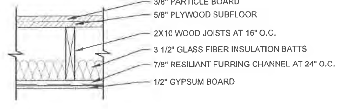
INFILL FLOOR FC 3242 - 1 HR. RATED STC 50
