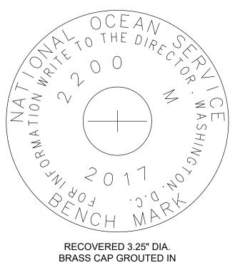
RECOVERED 3.25" DIA. BRASS CAP GROUTED IN CONCRETE FLUSH TO GROUND IN GOOD CONDITION.
