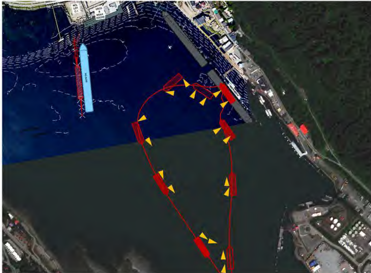
Maneuvers of Coast Guard 420-foot Coast Guard icebreaker HEALY to and from the Port of Juneau dock with two tugs assisting, with proposed HTD overlaid.
