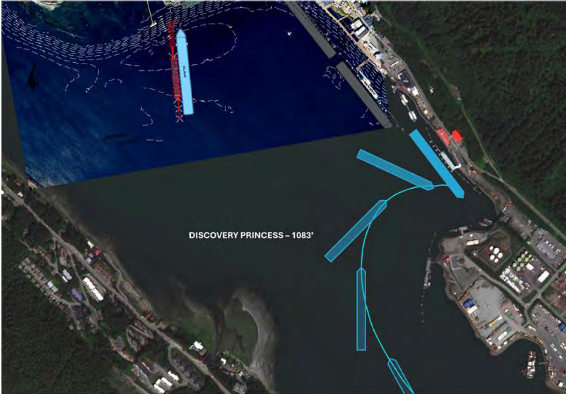
Figure (17). DISCOVERY PRINCESS arrival to Franklin Dock with overlay of the proposed HTD.
