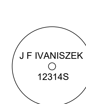
5/8" x 3/6" REBAR WITH RED PLASTIC CAP
