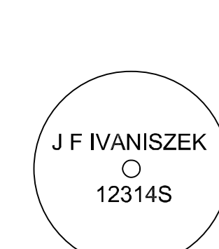
5/8" x 36" REBAR WITH RED PLASTIC CAP
