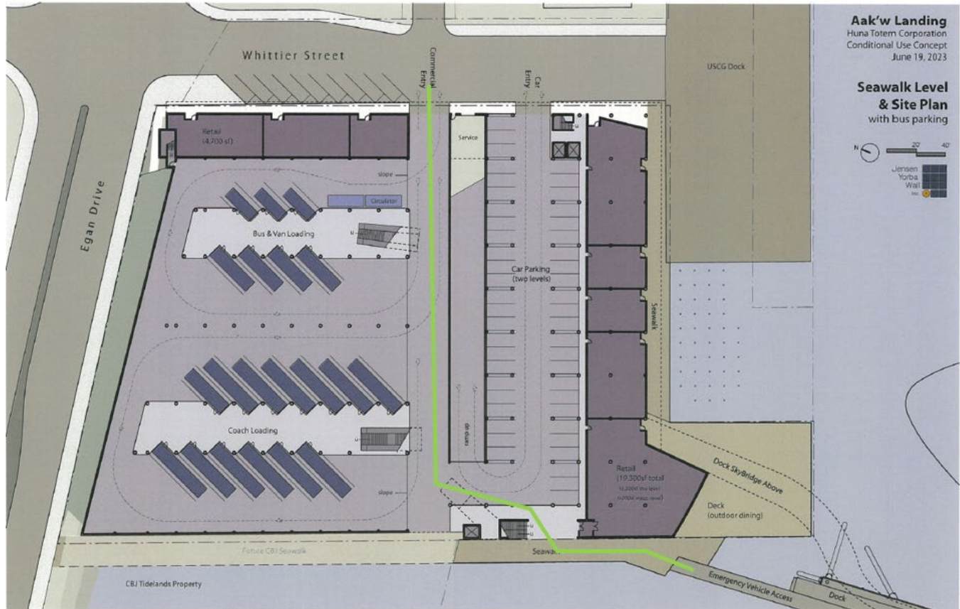
Figure 13: The green line shows ambulance access to the Emergency Vehicle Access. This route bypasses approximately 420 feet of seawalk along the waterfront, reducing conflict with pedestrians.
