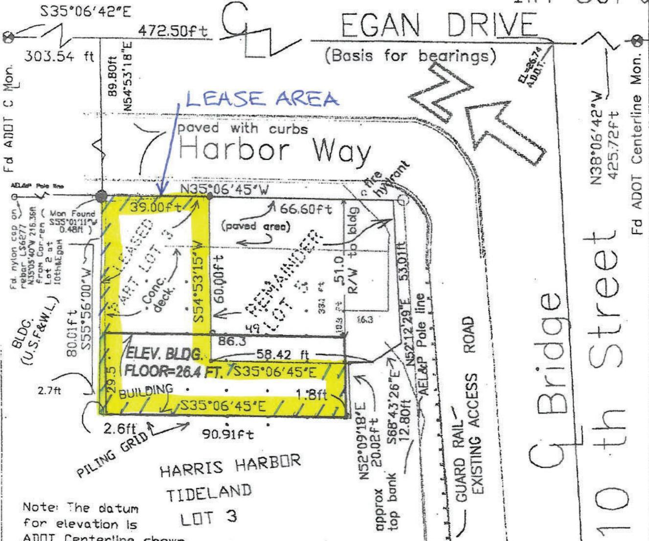
Note: The datum for elevation is ADOT Centerline shown based on USC&GS BM 15 EL=24.70 FT. above M.L.L.W.
