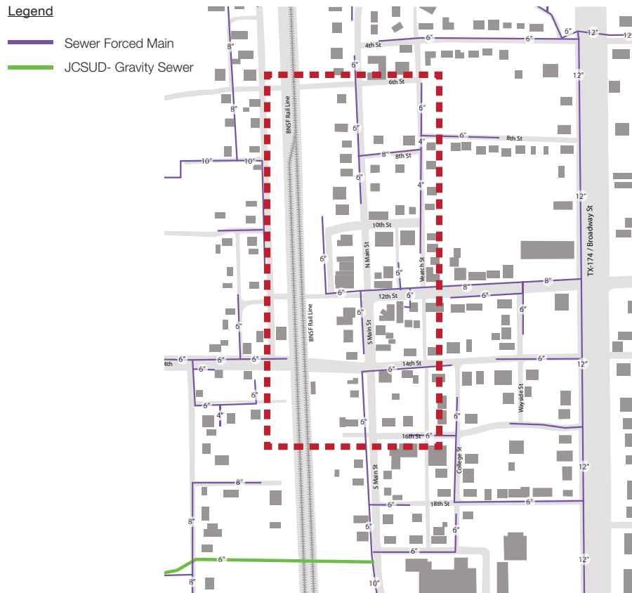
Figure 19: Existing Sewer Infrastructure Diagram
