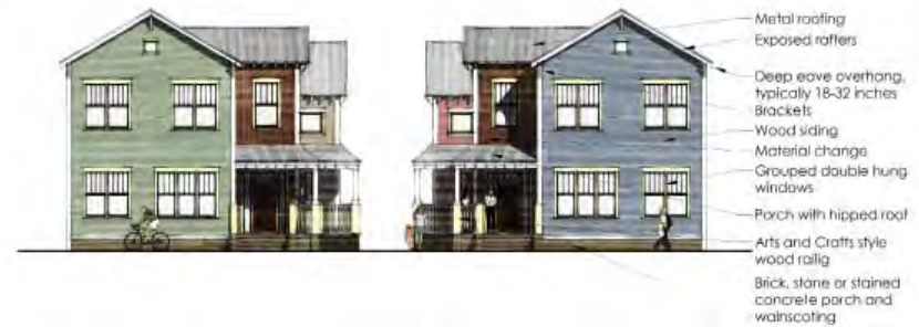
Figure 74: Cottage Court Medium Density Housing Elevation
