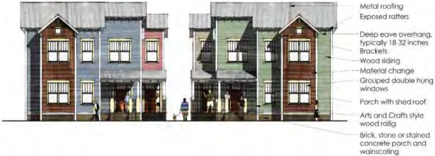
Figure 71: Cottage Cluster Medium Density Housing Elevation
