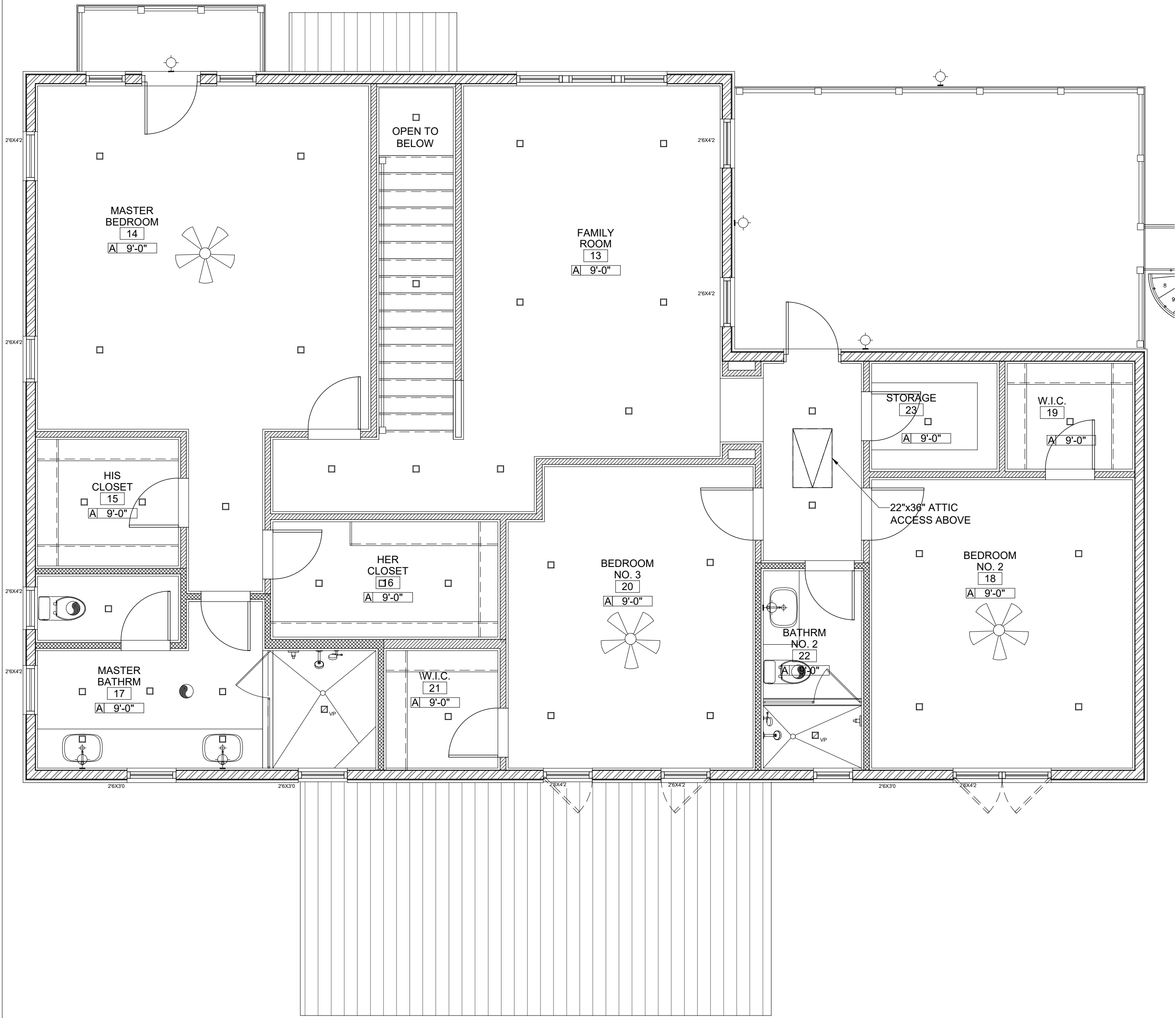
2 PROPOSED SECOND FL RCP SCALE: 1/4" = 1'-0"
