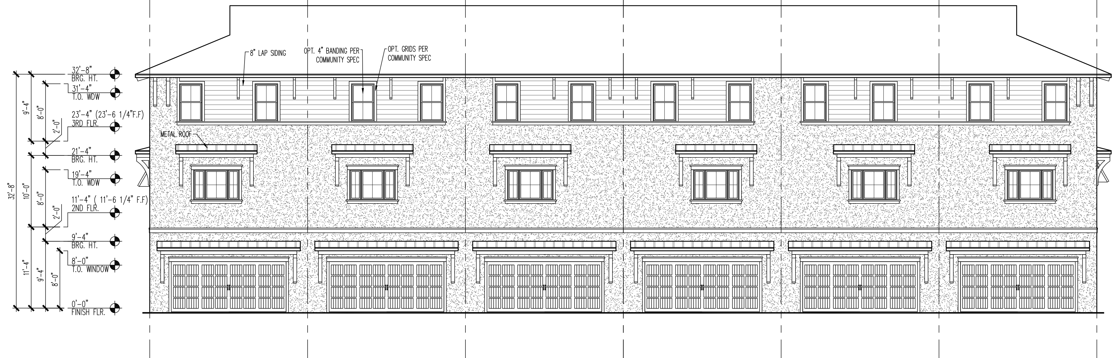
REAR ELEVATION-6-UNIT BUILDING
