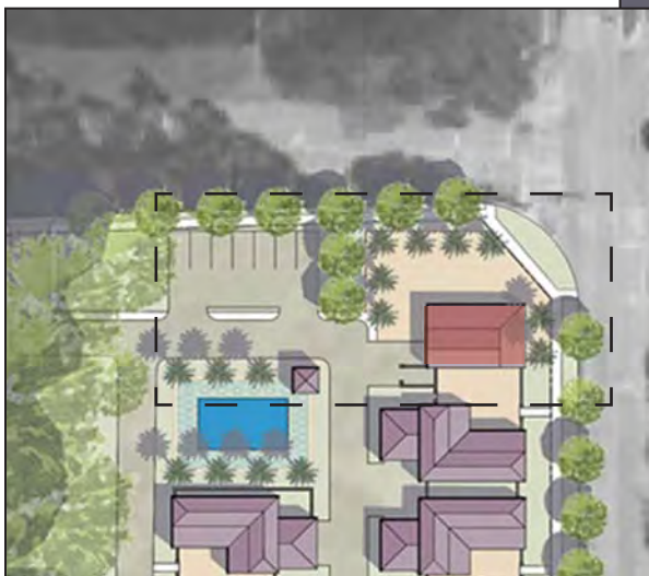
Top Right: A plan with 15 houses 2,700 SF each, with a site density of 5.9 du/ac.
