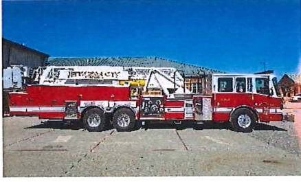
JCFD TRK 51- Aerial Ladder (2002 Ferrara Inferno) 2000 GPM Pump, 300 Gal Tank, 100' Aerial Platform
