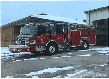
JCFD ENG 53 - Pumper (2019 Pierce Impel) 1500 GPM Pump, 750 Gal Tank
