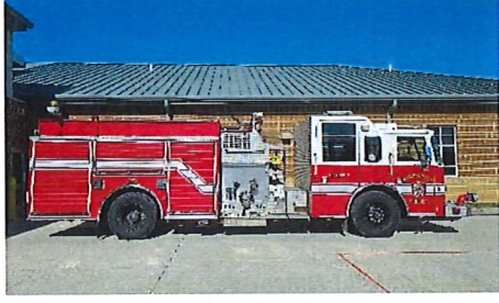
JCFD ENG 52 - Pumper (2003 Pierce Saber) 1500 PGM Pump, 1000 Gal Tank
