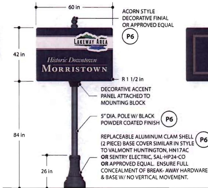
ELEVATION - G3.1 - Single Sided (Secondary Gateway) SCALE: 3/8" = 1'-0"
