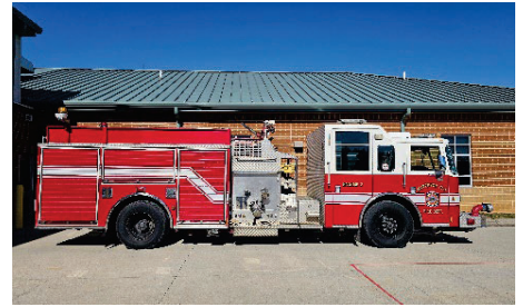
JCFD ENG 52 - Pumper (2003 Pierce Saber) 1500 PGM Pump, 1000 Gal Tank
