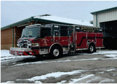
JCFD ENG 53 - Pumper (2019 Pierce Impel) 1500 GPM Pump, 750 Gal Tank
