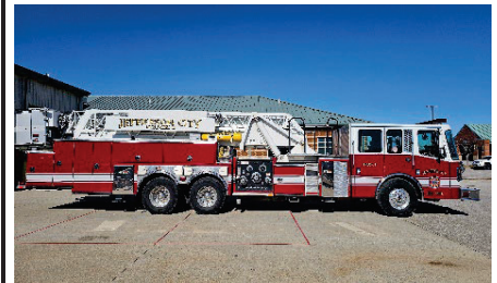
JCFD TRK 51- Aerial Ladder (2002 Ferrara Inferno) 2000 GPM Pump, 300 Gal Tank, 100' Aerial Platform
