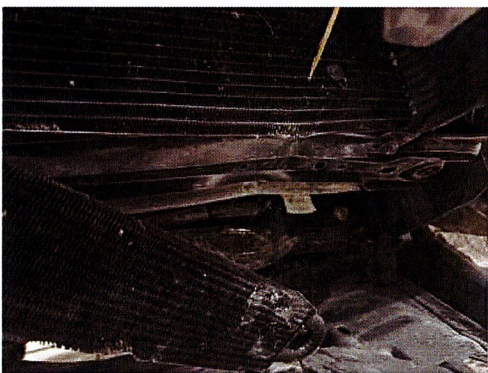
11/3/2025 Comments: POWER STERRING COOLER AND CENTER UNDERCOVER
