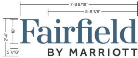
NON ILLUMINATED PIN-MOUNTED LETTERS SCALE: 1/2" = 1'-0"
