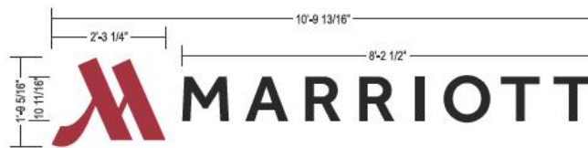
NON ILLUMINATED PIN MOUNT LETTERS DETAIL SCALE: 1/2" = 1'-0"
