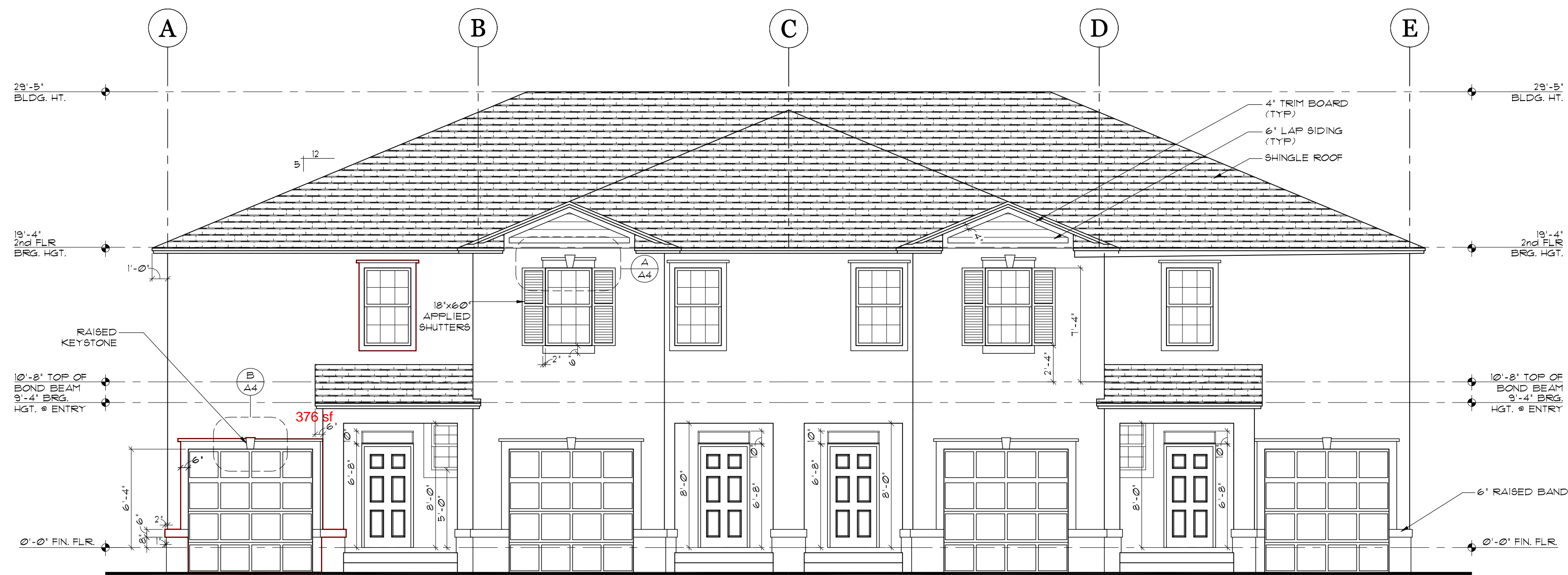
FRONT ELEVATION SCALE: 3/16" = 1'-0" TEXTURED FINISH NOTE: WALL PENETRATION FLASHING AS PER FBCR 103.4
