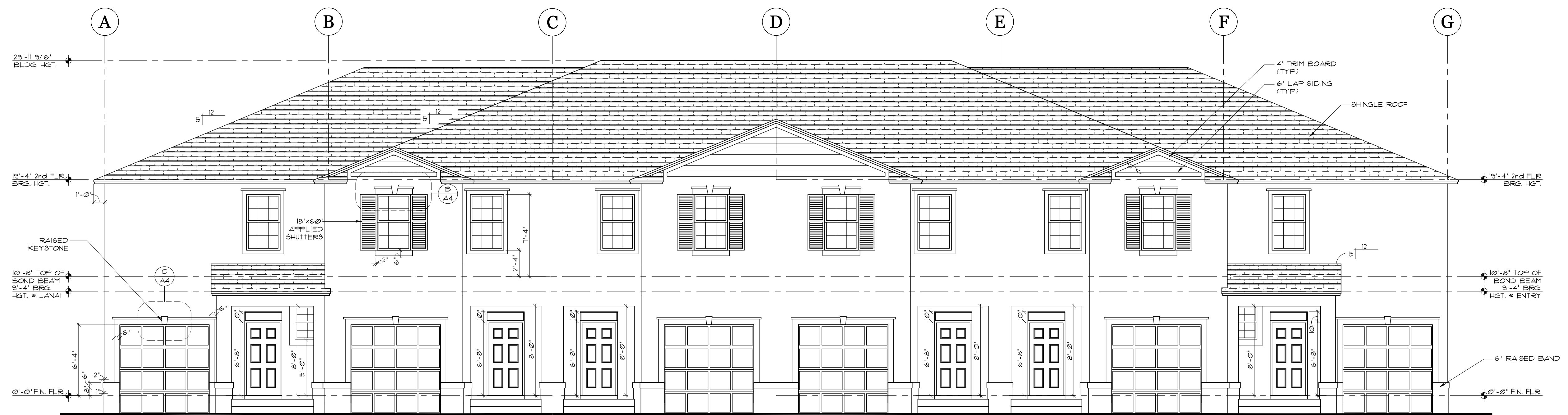
FRONT ELEVATION SCALE: 3/16" = 1'-0" TEXTURED FINISH NOTE: WALL PENETRATION FLASHING AS PER FBCCR 103.4
