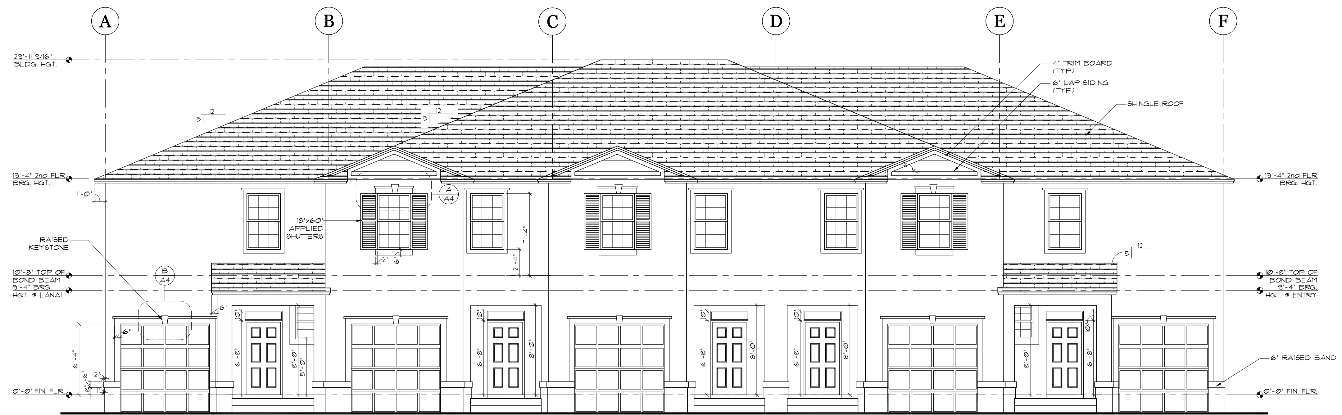
FRONT ELEVATION SCALE: 3/16" = 1'-0" TEXTURED FINISH NOTE: WALL PENETRATION FLASHING AS PER FBCR 103.4
