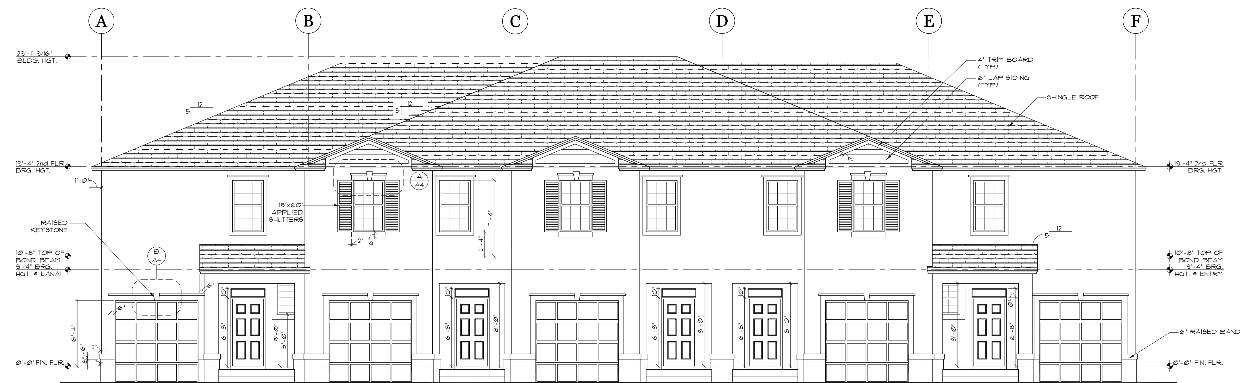
FRONT ELEVATION SCALE: 3/16" = 1'-0" TEXTURED FINISH NOTE: WALL PENETRATION FLASHING AS PER FBOR 103.4
