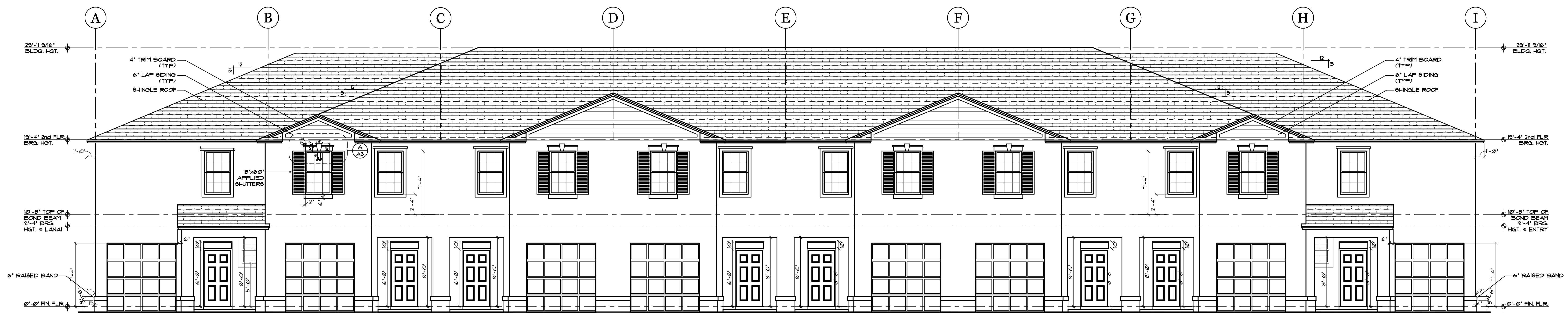
FRONT ELEVATION (LEFT) SCALE: 3/16" = 1'-0" TEXTURED FINISH NOTE: WALL PENETRATION FLASHING AS PER FBCR 103.4
