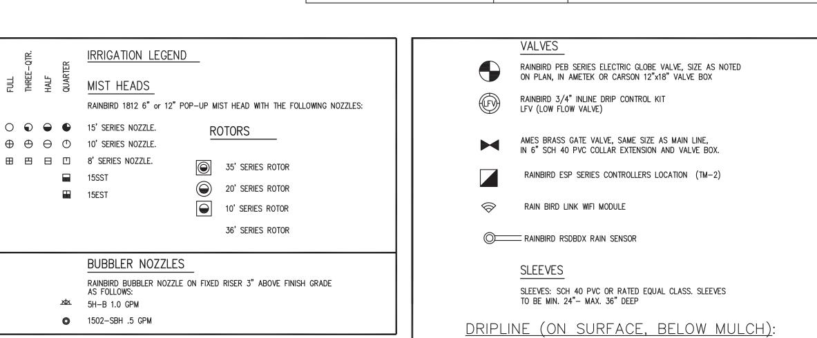
RAIN BIRD XFD DRIP LINE, 12" EMITTERS, .9 GPH EMITTERS XFD-09-12-100, XFD-09-12-250, XFD-09-12-500
