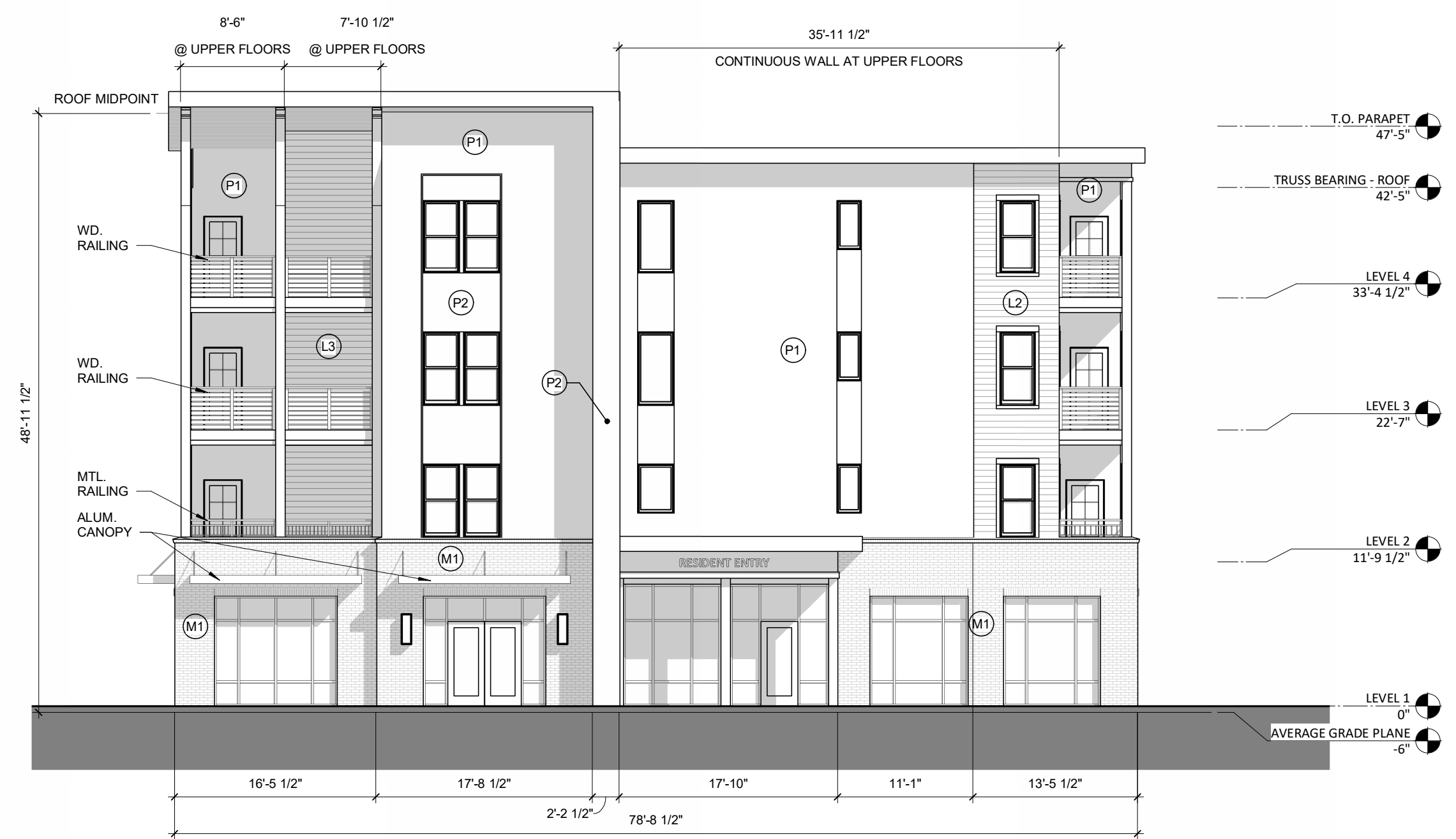
2 NORTH ELEVATION - LEASING ENTRY SCALE: 1/8" = 1'-0"
