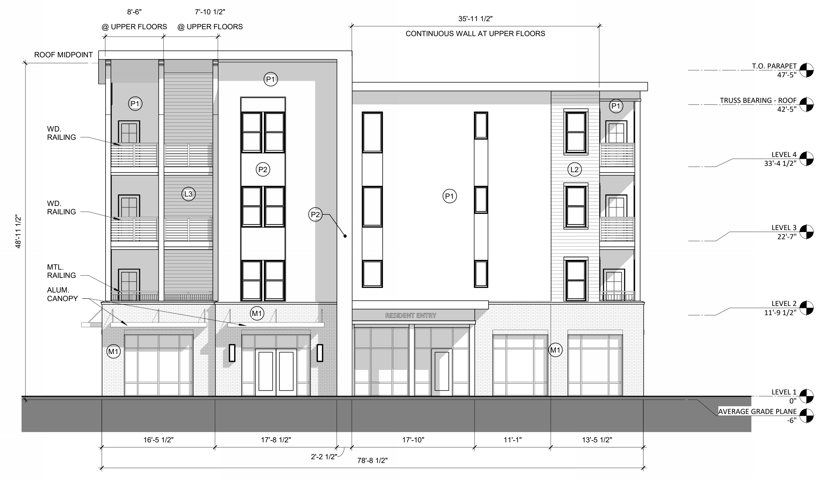
2 NORTH ELEVATION - LEASING ENTRY SCALE: 1/8" = 1'-0"
