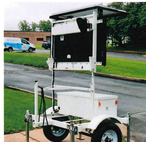
Flock-ready trailer with SpeedAlert 24 radar message sign and Flex LPR camera
