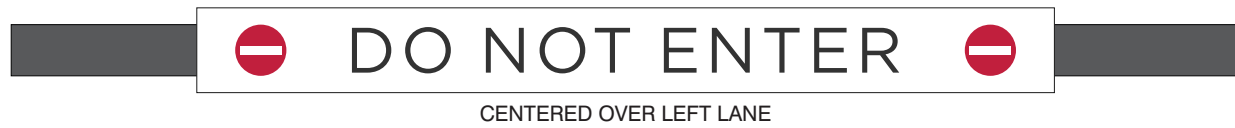
2 Front View @ Locations 1008, 1011, & 1029 Mounted 8'-2" from Grade Scale: 1:15
