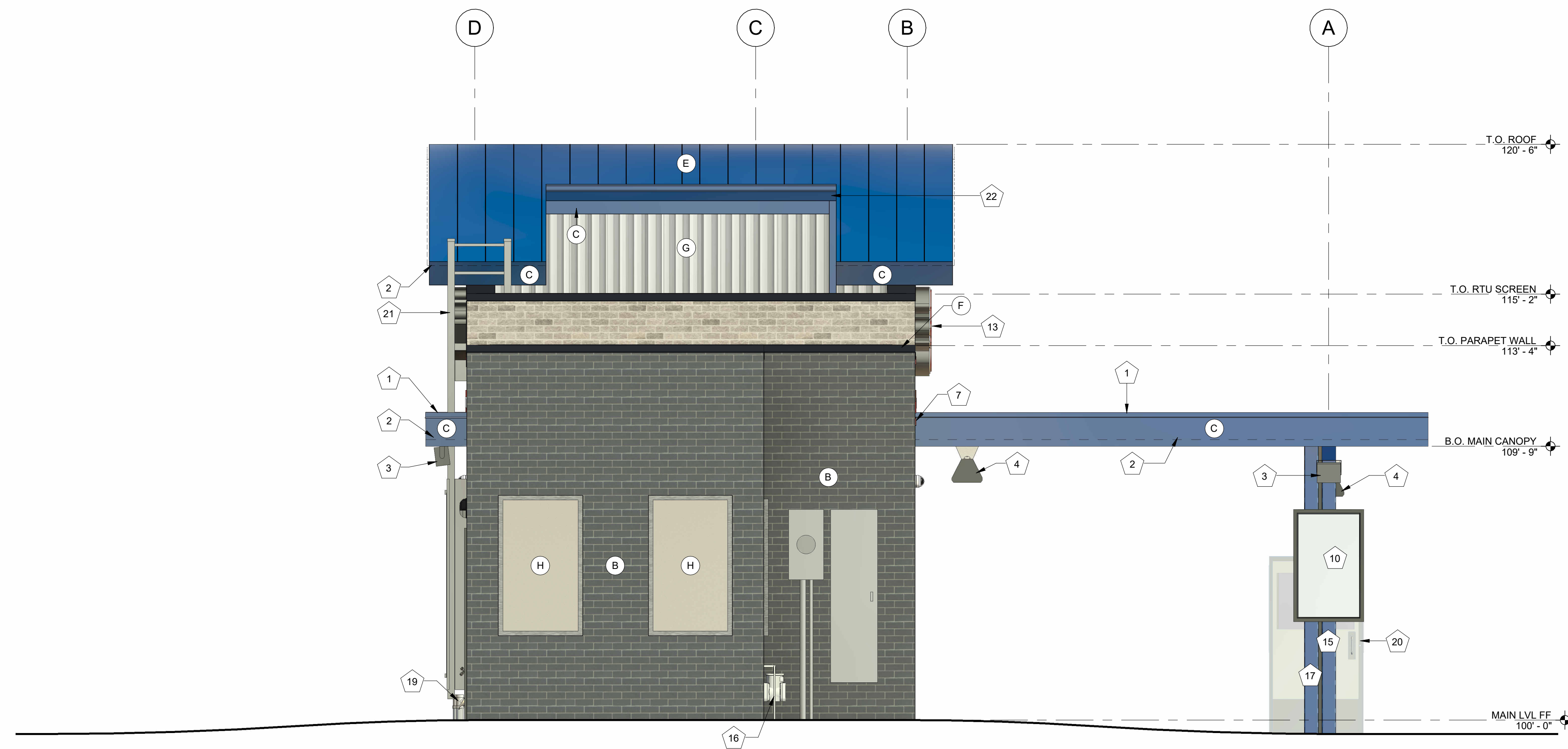
1 EXTERIOR ELEVATION - NORTH 3/8" = 1'-0"
