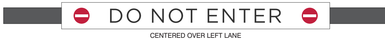
2 Front View @ Locations 1008, 1011, & 1029 Mounted 8'-2" from Grade Scale: 1:15
