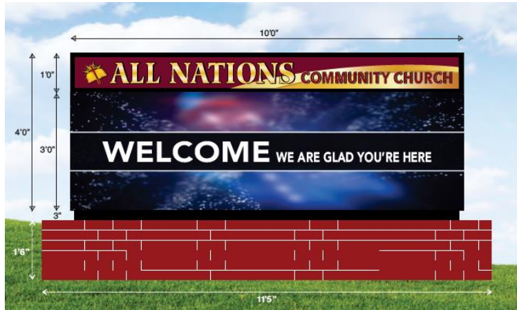
Figure B: Inset of design of proposed signage. Signage to be repeated twice to create V-pattern with monument signs at 60 degree angle.
