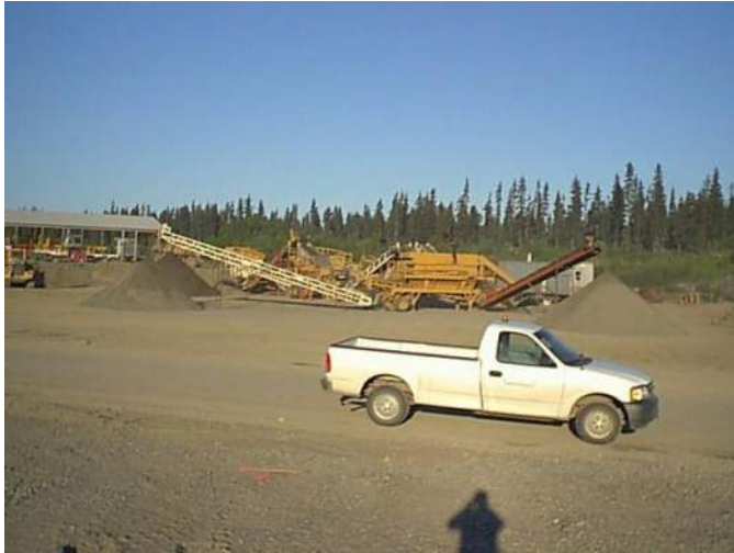
Photo 26: Crusher in operation at Brown's Pit. Production of aggregates for asphalt began on Thursday afternoon. Hot mix rock is being produced despite the fact that no base course has been crushed yet due to the lead time necessary for the mix design. (7/2/99)
