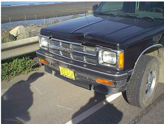
Photo 8: Front-end damage to 1993 Chevy S-10 truck caused by belly dump, morning of 6/24
