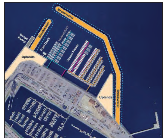
Port expansion adds a new basin with its own entrance adjacent to the existing Small Boat Harbor to relieve large vessel congestion in the small boat harbor, shown below.
