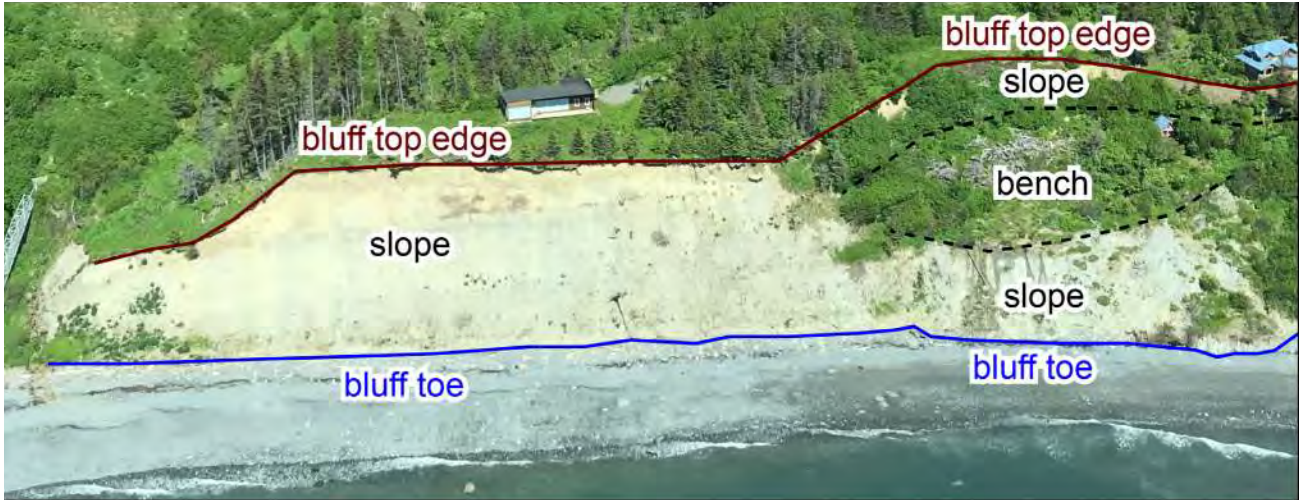
Figure 3. Oblique image of a coastal bluff with delineated toe (blue) and top edge (maroon). The right side shows how delineations are made for a complex section. The bluff has a bench (black dashed lines), so the delineated top edge is landward of this bench. In this example, there is a building on the bench that is seaward of the bluff top edge (far right side).
