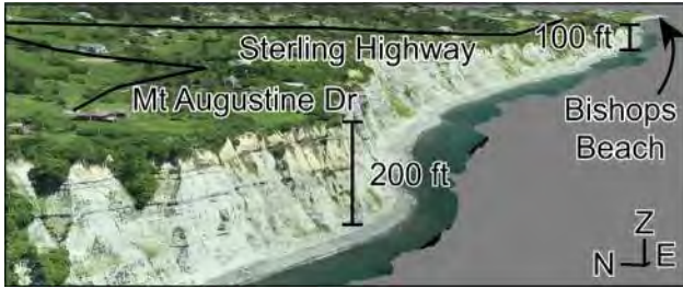
Figure 12. Looking east at the steep, exposed bluffs near Mount Augustine Drive in the oblique image-derived 3D model. The bluffs gradually shorten and become less steep toward Bishops Beach.
