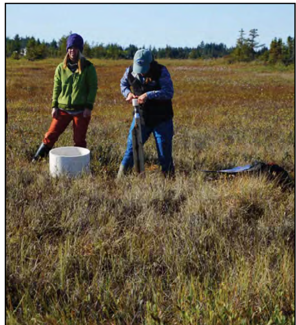
Testing peat depth in the Kachemak wetlands.
