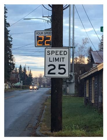
Figure 26: Speed Feedback Sign on Gillam Way in Fairbanks
