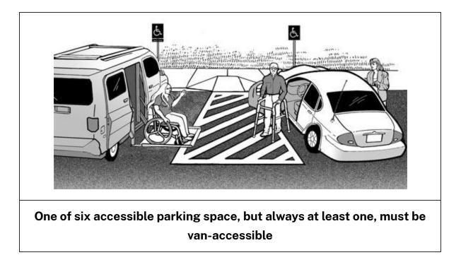
The required number of accessible parking spaces must be calculated separately for each parking facility, not calculated based on the total number of parking spaces provided on a site. One of six (or fraction of six) accessible parking spaces, but always at least one, must be van accessible.
