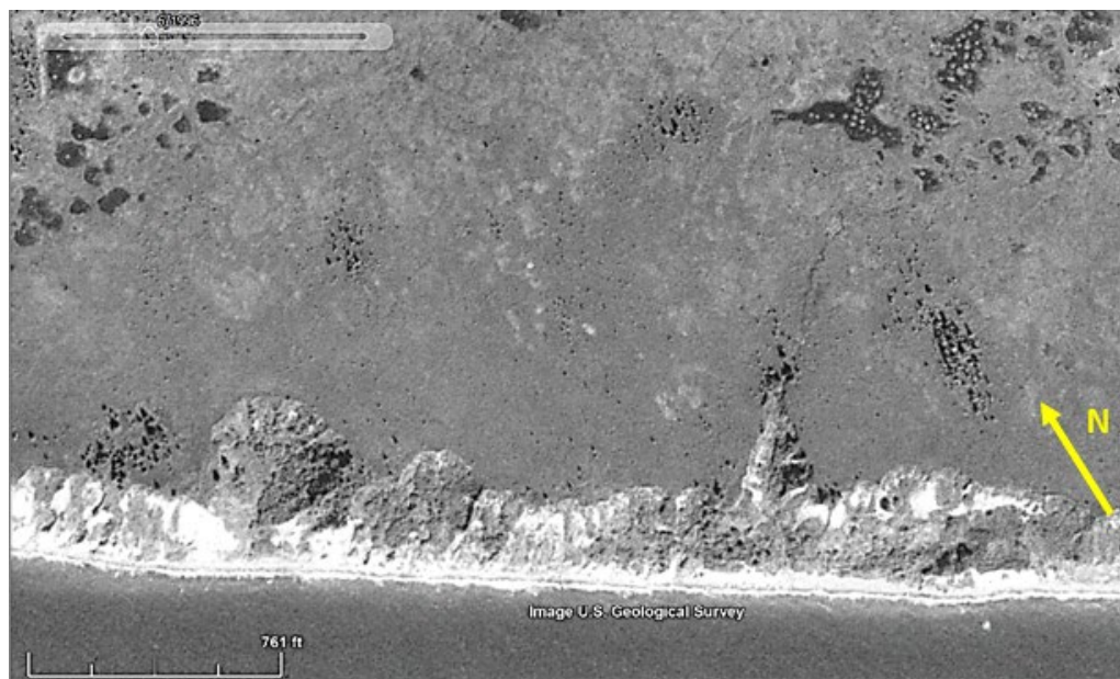
Fig. 7. Coastal bluff slumps along the coast north of Diamond Creek. Black areas are open water in wetlands. The bedrock of the Sterling Formation (mudstone, sandstone, and coal) forms the base of the bluff. Bluff height is ~1180 ft. Slumps are numbered northward from Diamond Creek (Berg 2024). The image is Google Earth 1996. The view is looking northeast.
