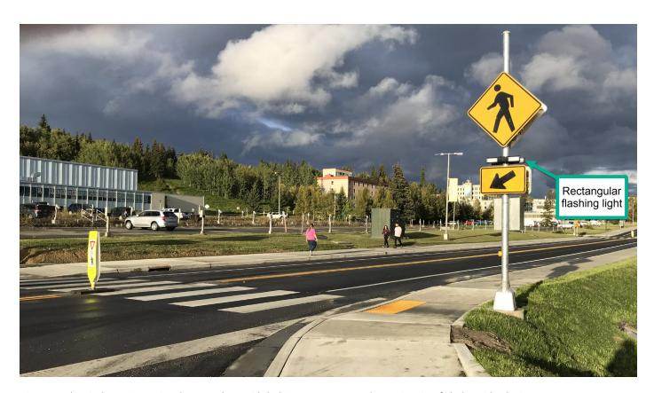
Figure 21: Electrical Warning Devices (Rectangular Rapid Flashing Beacon, or RRFB) on University of Alaska Fairbanks Campus
