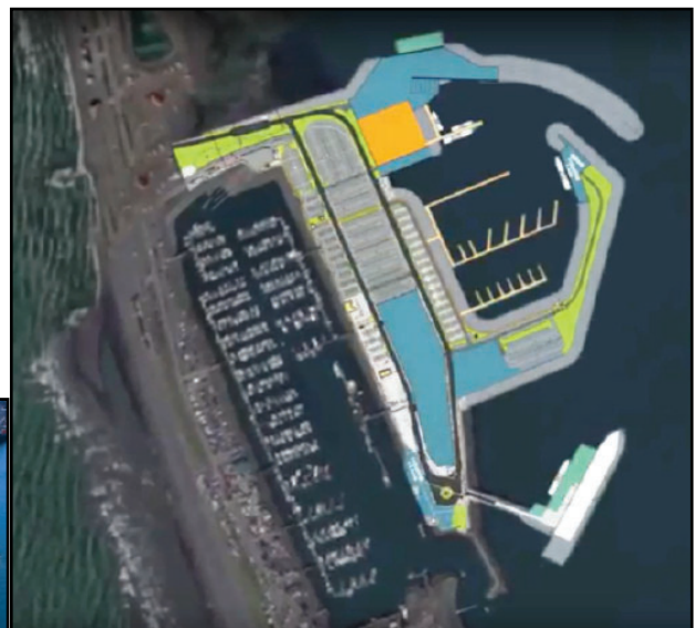
The large vessel port expansion adds a new basin with its own entrance adjacent to the existing Small Boat Harbor. It will relieve large vessel congestion in the small boat harbor and will provide secure moorage compatible with the USCG’s assets .
