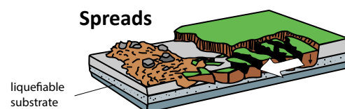
Figure 2. Types of slope failures as classified by Varnes (1978). Illustrations modified from Cruden and Varnes (1996) and Highland and Johnson (2004).
