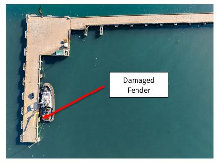
approximately 30,000 lbs. The fender system is designed to slide overtop of two pin piles that are driven into the seafloor and then are bolted to the dock face with brackets. Between the fender and dock are large rubber shock absorbers to assist with potential impact that can occur when a ship arrives at the berth.
