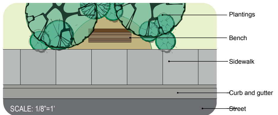
Least Preferred: Sidewalk adjacent to back of curb
