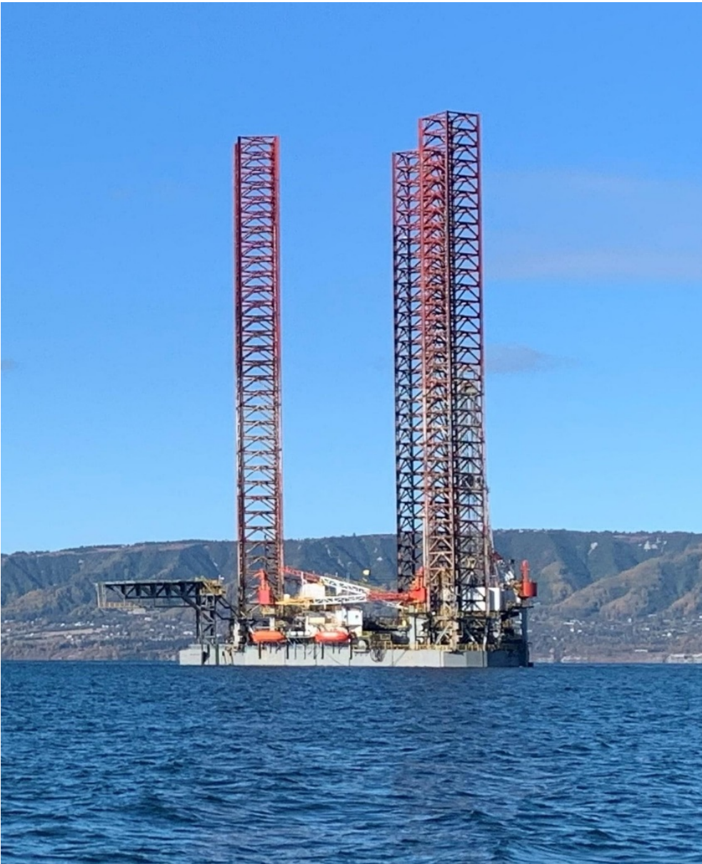
Jack-up drill rig Randolph Youst with its 400' legs fully elevated
