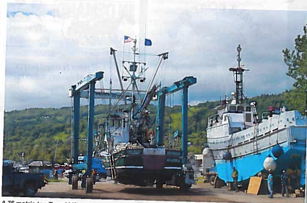
A 75 metric ton Travel Lift moves a commercial fishing boat from Northern Enterprises Boat Yard, across Kachemak Drive, to the dock for launching.
