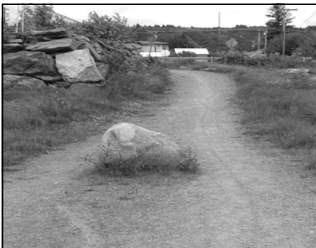
FIGURE D-17 Boulder used for access restriction.
