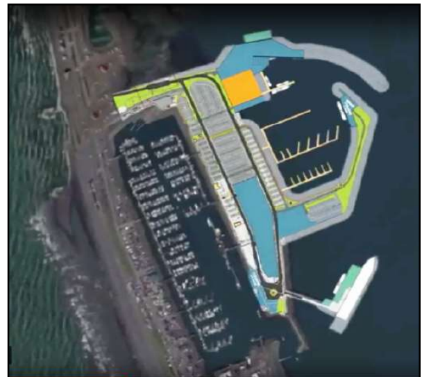
Port expansion adds a new basin with its own entrance adjacent to the existing Small Boat Harbor. It will relieve large vessel congestion in the small boat harbor and will provide secure moorage compatible with the USCG’s assets .
