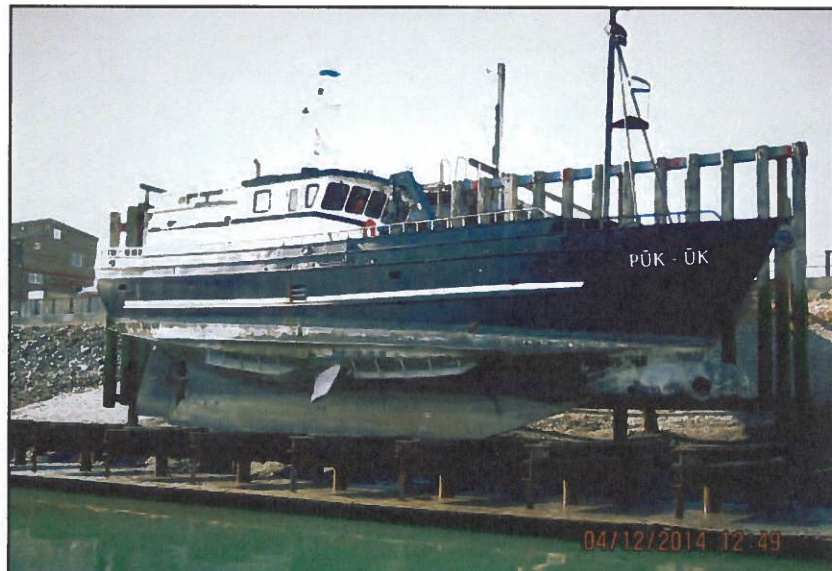
A marine vessel utilizing Homer Harbor's steel grid for repairs.
