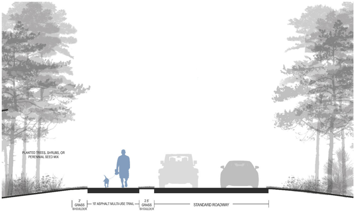
Proposed 10' Multi-Use Path next to Existing Roadway (Consistent with the Initial Report)
