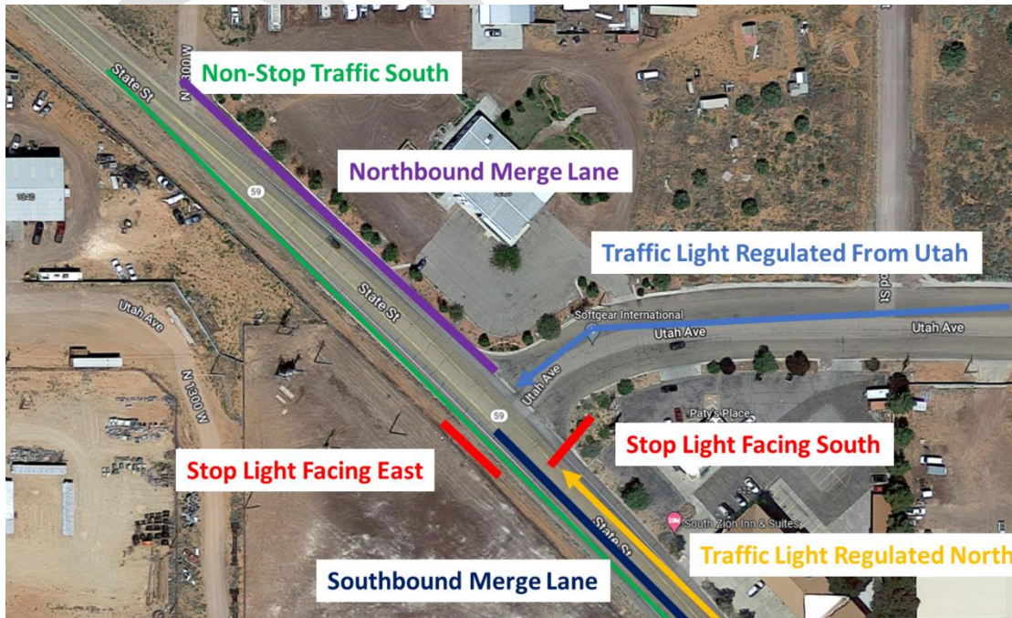
Figure 2 Concept of Intersection Widening
