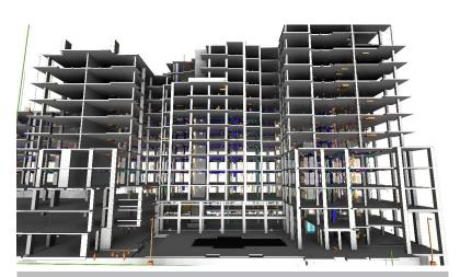
MEP coordination integrated with the structural model eliminates possible obstructions during construction.
