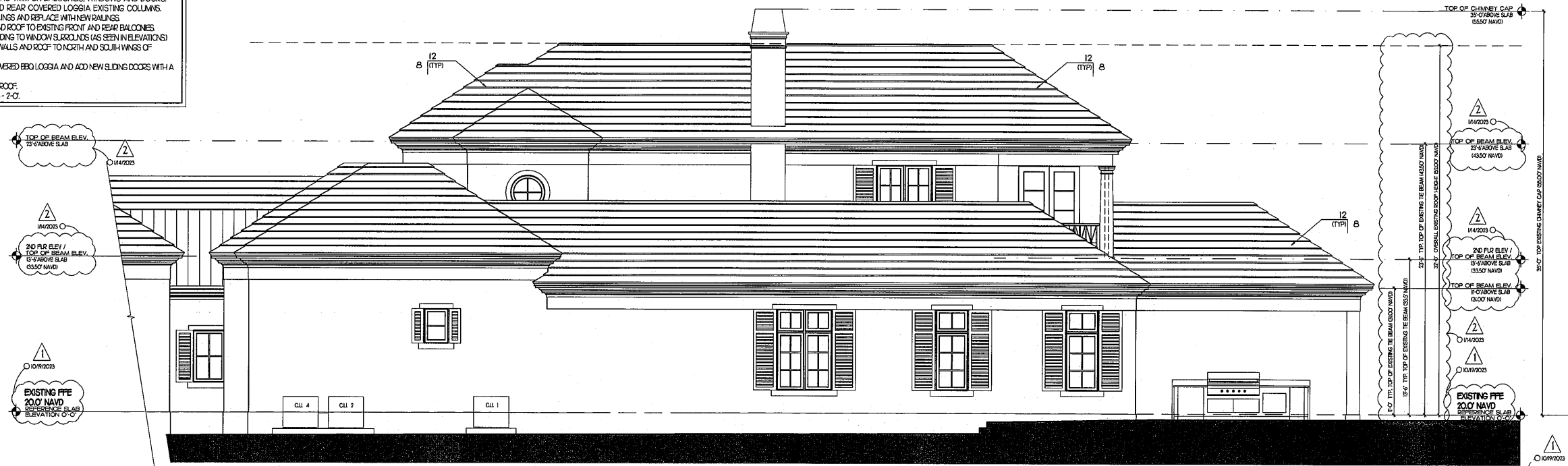
(EXISTING) MAIN HOUSE RIGHT ELEVATION 1/4" = 1'-0"
